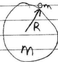
$$F_g = mg \quad \text{and} \quad F_g = \frac{GMm}{R^2}$$
