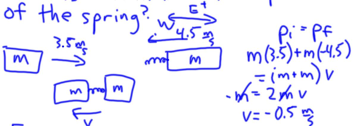
$$\begin{aligned} p_i &= p_f \\ m(3.5) + m(-4.5) &= (m+m)v \\ -10 &= 2mv \\ v &= -0.5 \frac{m}{s} \end{aligned}$$
