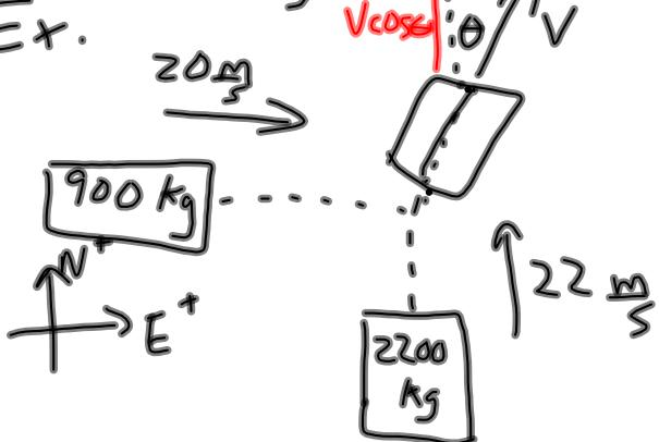
$$\begin{aligned} \vec{P}_i &= \vec{P}_f \\ N-S & \\ P_i &= P_f \\ (2200)(22) &= (2200+900) V \cos \theta \end{aligned}$$
